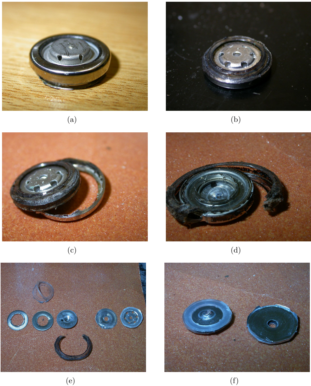
Figure 3.18: The Top Cap of a Panasonic 18650 Cell. (a) The top cap from top side; (b) the top cap from bottom side, rest from metal can removed; (c) top side, top of cap removed with grinder, pressure valve visible, plastic removed; (d) metal of top seal plate (figure 3.17 on page 34) weakened; (e) parts of the top cap, bottom the plastic removed in c, top the isolation between valve disc and circuit breaker, left to right: outer metal part of top cap – visible in a, PTC, valve disc, circuit breaker, inner metal part of top cap – visible in b; (f) pressure valve left and circuit breaker right.
